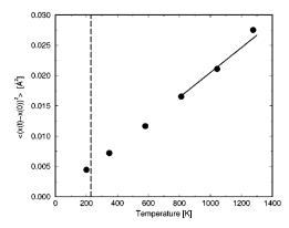
FIG. 2. Mean-square displacement for Nb atoms in  $Å^2$ . Dots are the molecular-dynamics (MD) simulations. Solid line corresponds to the quasiharmonic approximation. Classical MD is valid on the right of the dashed line and on the left side quantum effects are more important (Ref. 6).
