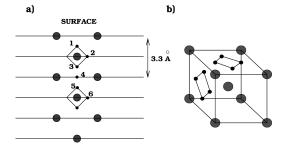
FIG. 1. (a) Cross section and (b) three-dimensional sketch of Nb (●) lattice with tetrahedral sites (•), the possible equilibrium location of the hydrogen atoms.
