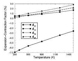
FIG. 3. Normalized change in lattice parameters for different layers of the Nb slab.
